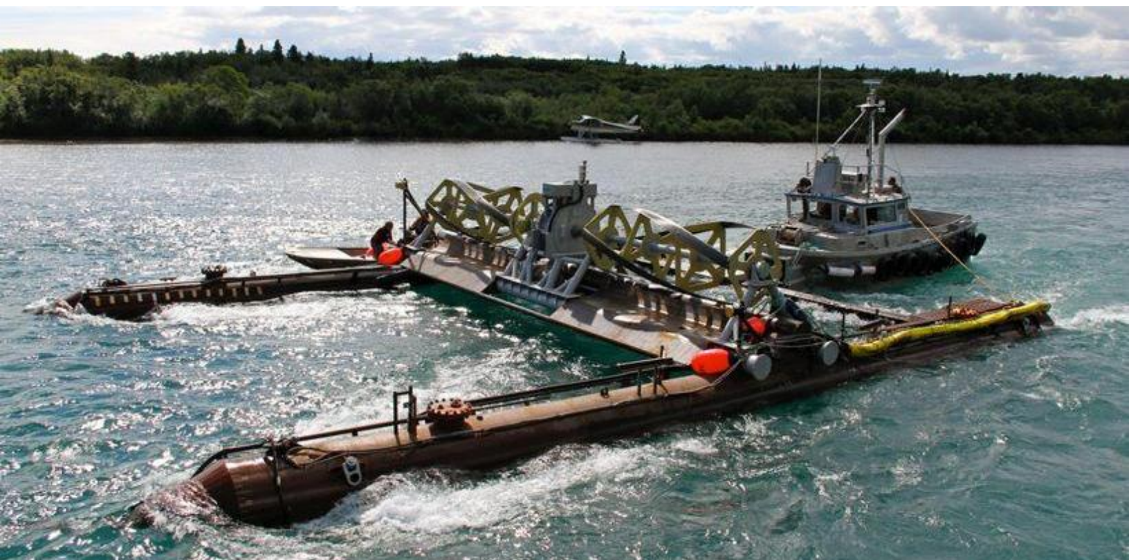
Figure 58: RivGen operating in the Kvichak River, near Igiugig, AK, in 2015 (ORPC) 58
